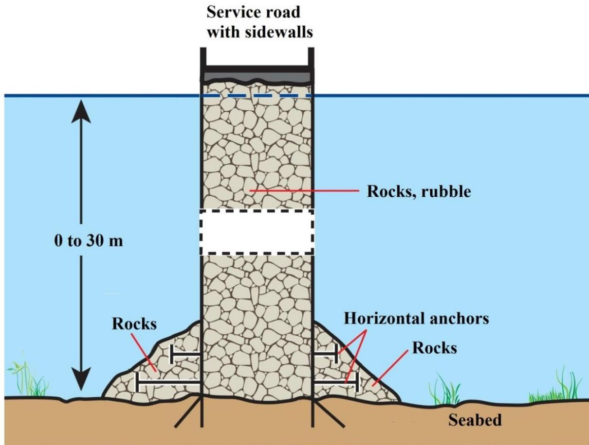
**Figure 16. Schematic cross section of a double-fence barrier with supply road between tsunami-flooding barrier and coast. The road has a width between 3 m and 5 m.**
