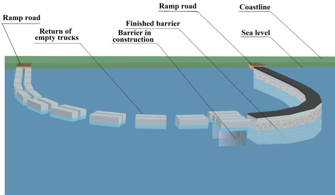
**Figure 10. Schematic view of double-pontoon bridge at the construction site, with finished tsunami-flooding barrier to the right. After delivery of steel fence and rocks, the trucks return to the coast on single-pontoon or on double-pontoon bridges to the left.**
