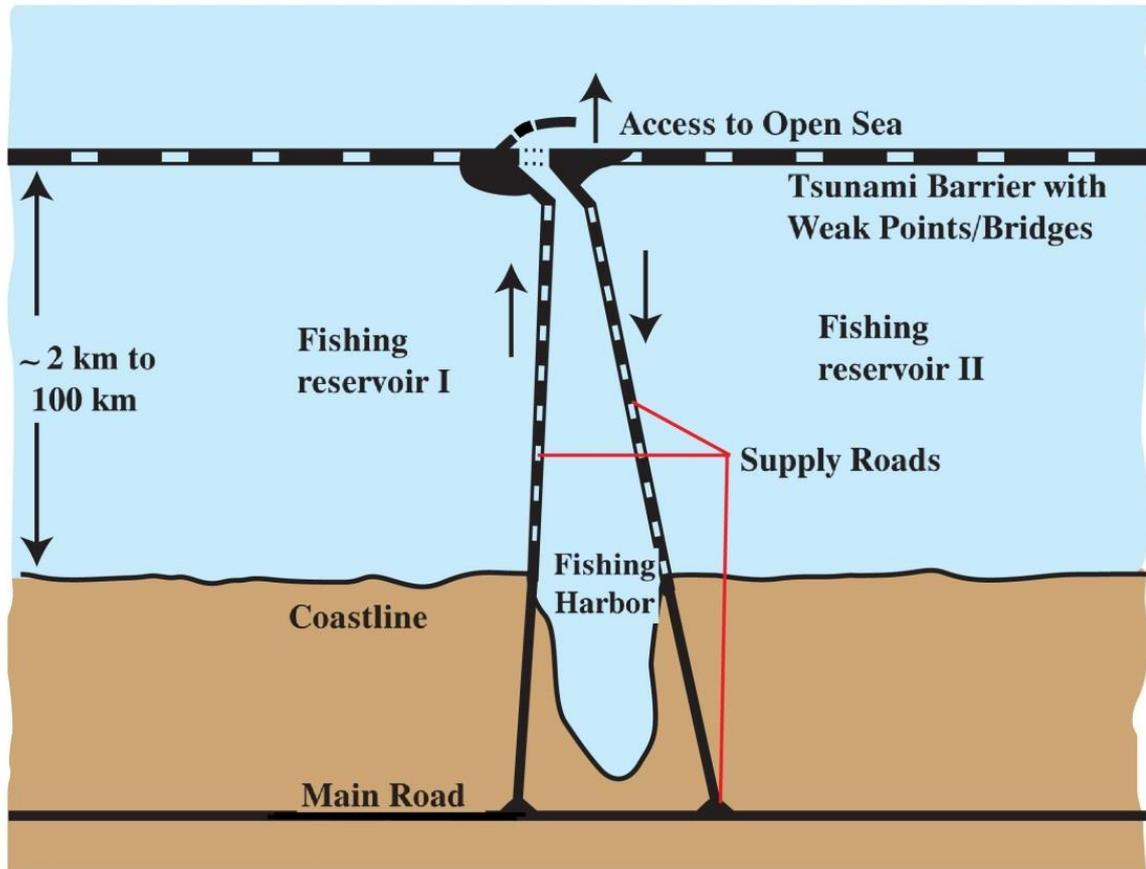
**Figure 15. Schematic top view of fishing reservoirs, supply roads, and of fishing harbor with access to the sea**
