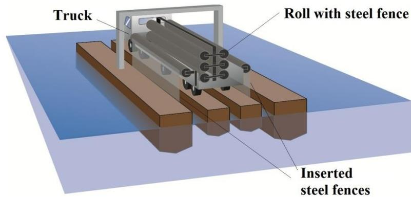
**Figure 9. Schematic view of a truck on a double-pontoon bridge simultaneously inserting two steel fences into the sea.**
