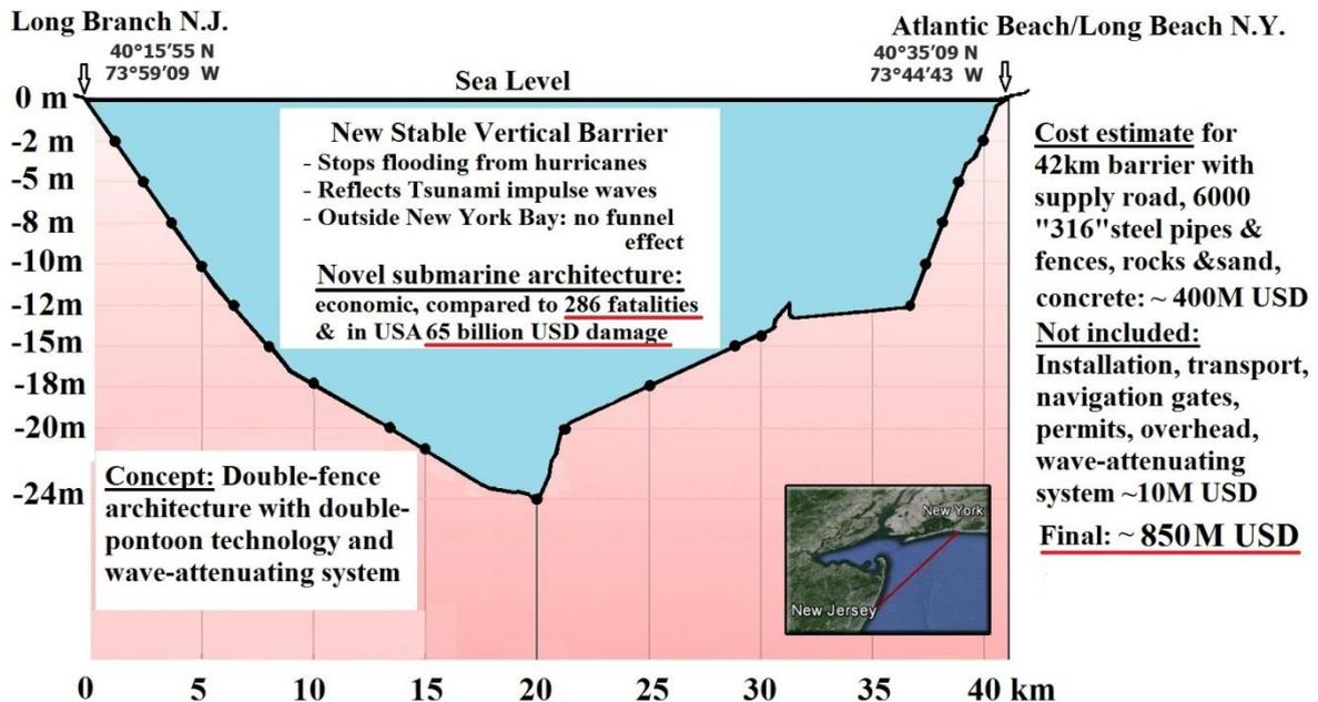
**Figure 13. Sea depth profile in front of New York bight with cost estimate for 42km tsunami-flooding barrier crossing the bight, where navigation gates are not included**
